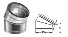
Use elbows to offset obstructions such as rafters, ridgepoles, or joists. 10"-16" DuraChimney II may have two pair of elbows, if needed. Offsets greater than 30° are not allowed. Elbows are not adjustable.
