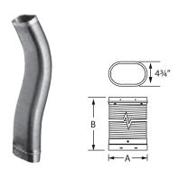
Use through damper and smoke shelf area. Built-in fittings. Use to connect from oval stove outlet to round DuraLiner. Use with DuraLiner Insulation Kit (ProMesh and ProFoil), where flex extends into clay liner, for zero clearance applications. Oval-to-Oval Flex pipe built from .016", 304 stainless steel, 4-ply construction.
