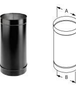
Use for a single-wall connector pipe. Requires 18" clearance to combustibles. Subtract 1 ¼" from length to calculate the installed length.
