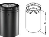
Use to add length to a straight length of DirectVent Pro. 8 ½" pipe adds 3"- 7" of length, 16" pipe adds 3"- 14 ½" of length, when used with rigid sections of pipe. Direct vent lengths feature a fully unitized, twist-lock construction. Use of sealant is optional, unless specified by the appliance manufacturer. Available in black or galvalume exterior (both feature laser-welded outer wall seams). Does not fit DirectVent GS pipe.
