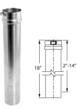
Use to add length to straight length of FasNSeal pipe. Adds 2"–14" of length. Requires at least 4" overlap for a secure connection. **Available in Custom Lengths.**
