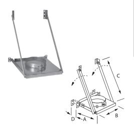
Supports the chimney at the base of the installation or along a wall or other vertical surface serving as an intermediate support. Also permits the tee to be installed above or below the support. It comes with a tightening collar locked around the chimney and secured by two self-tapping screws (included). The collar rests on a horizontal plate. When used as a base support, it lends itself to the addition of an insulated tee cap. Refer to chart for loadbearing capacity.
