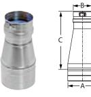
Use to reduce vent diameter. Creates a smooth transition for an undisruptive flow. Additional sizes available, but reductions are limited to a maximum of 2" reduction in diameter.
