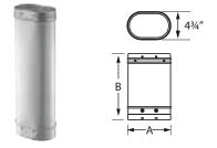
Use to reline masonry chimney with 0/0 clearance. Available in oval 6" and 8" diameters; 12", 24", 36", and 48" lengths. Factory-insulated. Built-in, pre-drilled fittings for riveting joints. 304 stainless steel inner and aluminized steel outer. Note: to calculate the installed length of 5", 6", and 8" DuraLiner pipe subtract 1 ½" from each joint overlap of liner pipe sections.
