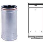
Features fully unitized, twist-lock construction in 3" diameters. It can be used in both vertical and horizontal installations. Stainless steel welded seam inner wall, combined with a galvalume weleded seam outer wall. Inner and outer are sealed with O-Ring gaskets. Galvalume or painted black outer finish. To calculate installed length, subtract 1 1/2" from each length of pipe.
