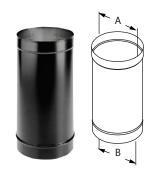
Use for a single-wall connector pipe. Requires 18" clearance to combustibles. Subtract 1 ¼" from length to calculate the installed length.
