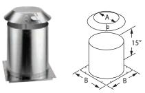
Required for installations that pass through an attic to prevent insulation and debris from accumulating near the chimney. Fits over Firestop Radiation Shield or a support box. Consists of two parts – a collar and a base.
