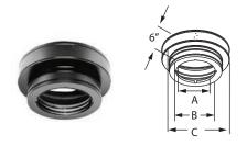
Supports chimney pipe and provides a positive connection between support box and chimney with a built-in twist-lock. Supports up to 60' of DuraTech Chimney. Use adapter to attach DVL or DuraBlack to the support box. Painted black. Trim collars are sold separately. (For adapters see DVL/DuraBlack section).
