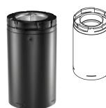
Designed for appliances tested and listed for direct vent. Features a fully unitized twist-lock construction in both 4" x 6  $\frac{5}{10}$ " and 5" x 8" vent sizes. Use of sealant is optional, unless specified by the appliance manufacturer. To calculate install length, subtract 1  $\frac{1}{2}$ " for each joint. No beads or hems. Black pipe lengths feature exterior laser-welded seams.
