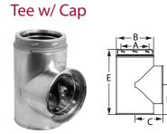
Use for through-the-wall installations. Includes removable tee cap for easy chimney cleaning or inspection. Wall Straps, a Wall Thimble, and an Adjustable Tee Support Bracket must be installed with the Tee as directed. Available in stainless steel or with a galvalume outer wall and stainless steel inner wall. See installation instructions for proper location and installation of Tee.
