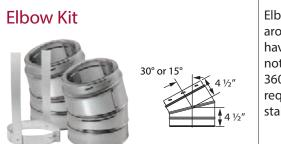
Elbow Kit includes: 2 Elbows and 1 Elbow Strap. Use for offsets around obstructions such as rafters, ridgepoles, or joists. May have two pairs of elbows, if needed. Offsets greater than 30° are not permitted in accordance to UL 103 standards. Elbows swivel 360° at base (angles are not adjustable). A pair of elbows is required to return an offset chimney back to vertical. Available in stainless steel (5"-8" SS) or galvalume (6"-8" GA) outer wall.
