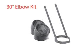
The 8" DuraChimney II Elbow Kits include 2 elbows and 1 elbow strap. Use to offset around obstructions such as rafters, ridepoles, or joists. Offsets greater than 30° is not allowed. Elbows are not adjustable.
