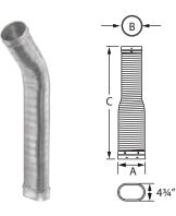
Use through damper and smoke shelf area. Use to connect from oval stove outlet to round DuraLiner. Use with DuraLiner Insulation Kit (ProMesh and ProFoil), where flex extends into clay liner, for zero-clearance applications. Built from 1-ply construction, .005" 304 stainless steel.
