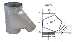
Use in place of any tee for a 45° angle instead of 90°. The branch has a smaller diameter, so it can be used to increase to a larger diameter as a manifold connection to gang multiple boilers into a common vent. Maximum diameter increase is 6". Available in custom size combinations.
