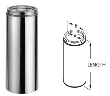
To calculate installed length of 5", 6", 7", or 8" DuraTech Chimney, subtract 1 ¼" from each joint overlap of chimney pipe. Allow a minimum of 2" air space to combustibles when installing DuraTech Chimney.
