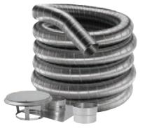
Kit includes: Top Plate with welded Storm Collar, and Cap, plus DuraFlex SS Connector, and DuraFlex 316 length. Flex remains secured to the Storm Collar/Top Plate when removing the cap section for inspections and cleaning.
