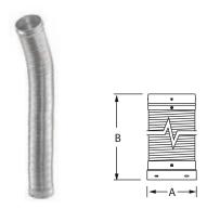
Use through damper and smoke shelf area. Use with DuraLiner Insulation Kit (ProMesh and ProFoil), where flex extends into clay liner, for zero-clearance applications. Built from 1-ply construction, .005" 304 stainless steel.
