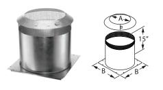
Use in installations that pass through an attic to prevent insulation and debris from accumulating near the chimney, unless chimney is enclosed through attic. Fits over Firestop Radiation Shield or a support box. Consists of two parts - a collar and a base. Mesh sleeve around top.
