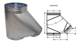
Use in place of any tee for a 45° angle instead of 90°. The branch has a smaller diameter, so it can be used to increase to a larger diameter as a manifold connection to gang multiple boilers into a common vent. Maximum diameter increase is 6". Available in custom size combinations.
