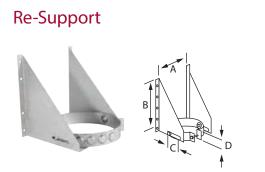
Use to support the chimney on a vertical wall. The triangular plates allow a 2" to 4" lateral adjustment of the support to the vertical surface. This support can also be used as a wall support above the insulated tee or as a support for an offset elbow. Refer to chart for loadbearing capacity. In shorter chimney stack applications, the Re-Support can also be used in place of a Tee Support. Universal design works with 6", 7", or 8" pipe diameters.
