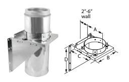
Use as wall support for chimney system. Use of straps is optional. Supports up to 50' of DuraTech Chimney without straps, and 70' of DuraTech Chimney with straps. Attaches to chimney pipe. Can be installed above or below the Tee. If installed below the Tee, a short section of pipe is required. Adjustable base provides 2" to 6" clearance to wall.
