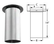
Use to adapt DuraBlack pipe to ceiling support box or finishing collar. Adds 3" - 13" of length to rigid pipe. Allows drip-free installation without cutting the pipe. Can be used in line to create a telescoping combination when used with a straight length of pipe.
