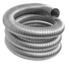
Used to line masonry chimneys venting Category I, natural gas, propane, furnaces, space and water heaters. Single-wall, .006" AL29-4C stainless steel. Continuous weld construction. Custom lengths available using XX stock#'s. (e.g.: For a 7" diameter, 40' length stock# would be QTY 40 of 7VG-XX). Maximum length of 150' for 3" - 9" diameter custom orders and 25' for 10"-12" diameter custom orders. Must be ordered in 10' increments.
