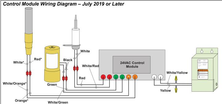
\* NOTE: The thermopile must connect to the control module as shown above (white/orange wire connects to the white thermopile wire and orange wire connects to red thermopile wire). Do not reverse the wires. If the wires are reversed, the torch will not work correctly.
