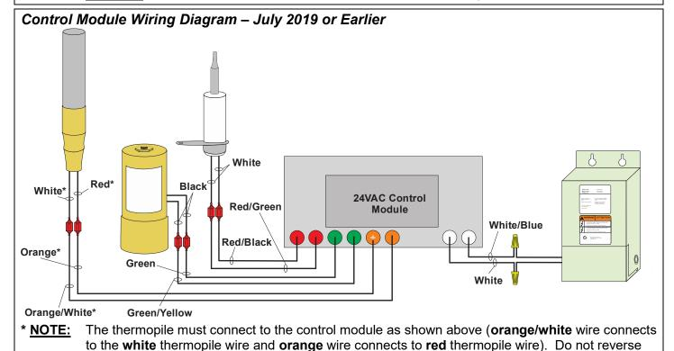
the wires. If the wires are reversed, the torch will not work correctly.
